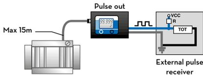
Display pulse transmitter externally powered
